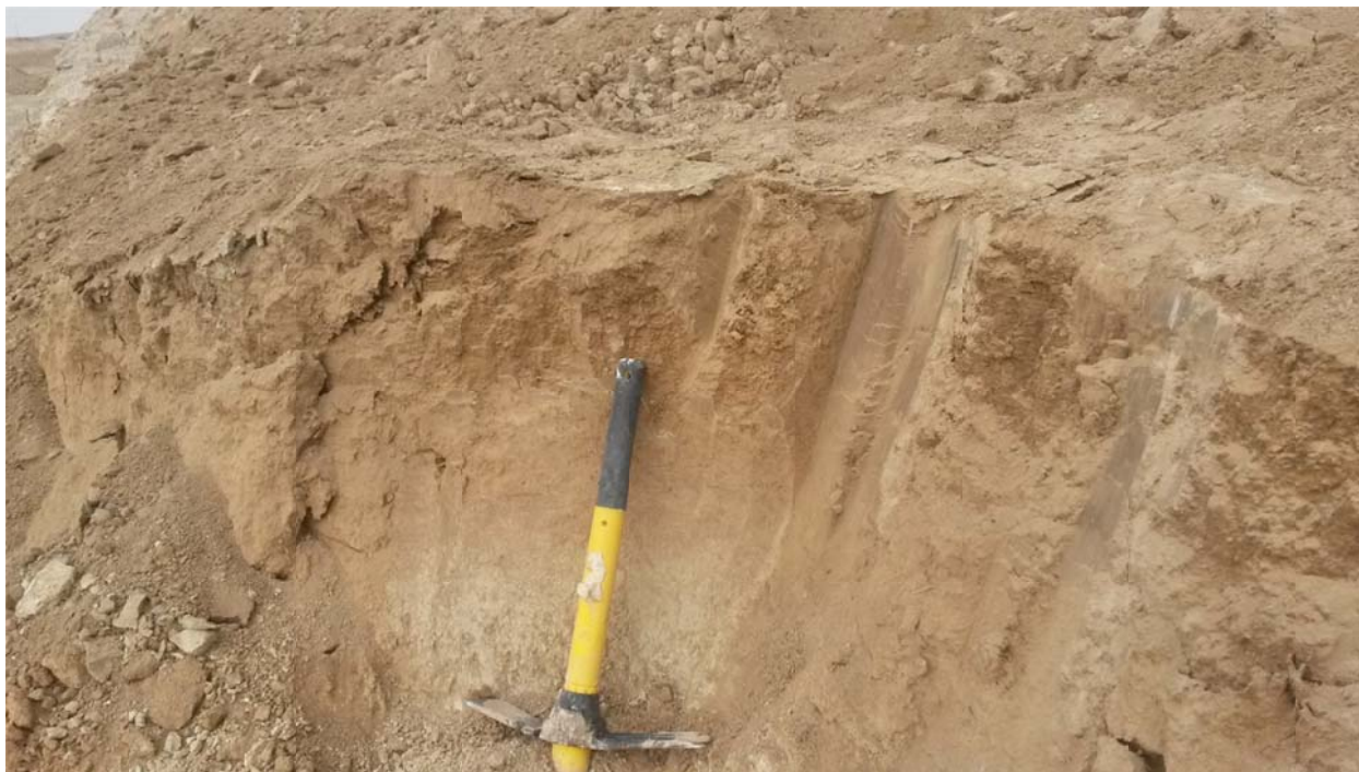
Figure 5. An example of upper soil-modified eolian silt in Pit 29. Basal contact of the silt is approximately located at the middle of the pick handle. It is a gradational contact between eolian silt intermixed with regressive Lake Bonneville marl (bottom of the pick handle).
